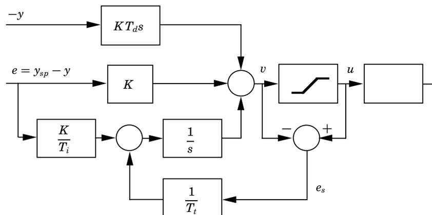
The signal  $e_s$  is fed to the input of the integrator through gain  $1/T_i$ . The signal  $e_s$  is zero when there is no saturation. Under these circumstances it will not have any effect on the integrator. When the actuator saturates, the signal  $e_s$  is
